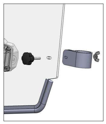
2. Snap 4 P Clamps onto the roll cage in the approximate locations of the mounting holes in the windshield. Mount windshield with the 4 threaded knobs and wing nuts. Move windshield around as necessary for alignment before fully tightening.
